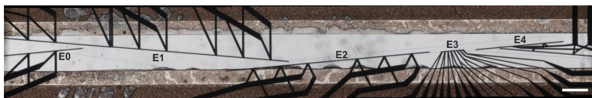
Figure 19: Microscopic image of the PROC2 main channel. Electrodes are labelled according to the main text. The scale bar represents 500 \mu\text{m} .
