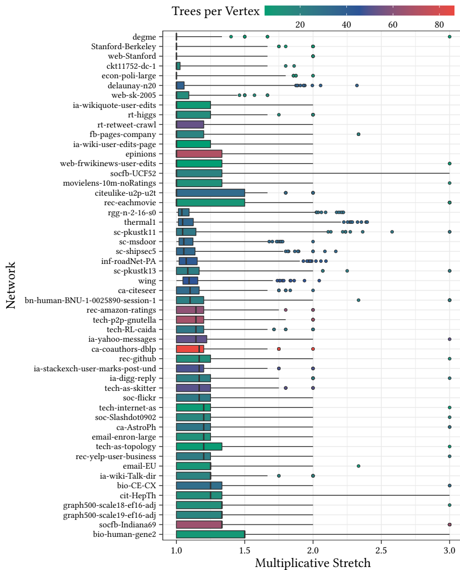
Figure 4.4: Multiplicative stretch when routing with a tree-cover obtained using the PROTON algorithm with a = b = 2 . Colors show the number of trees k that an average vertex is contained in. The boxes denote the interquartile range extending to the 25th and 75th percentile with horizontal bars showing the median. Whiskers extend to 0.1% and 99.9%, while circles show values beyond that.
