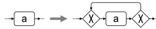
Fig. 6.9. Insertion of a XOR-bordered cyclic bond for an activity with interleaving order as a self-relation.
