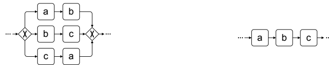
(a) The fragment fulfills the constraints a \rightsquigarrow b , b \rightsquigarrow c , and c \rightsquigarrow a at the expense of activity duplication.
