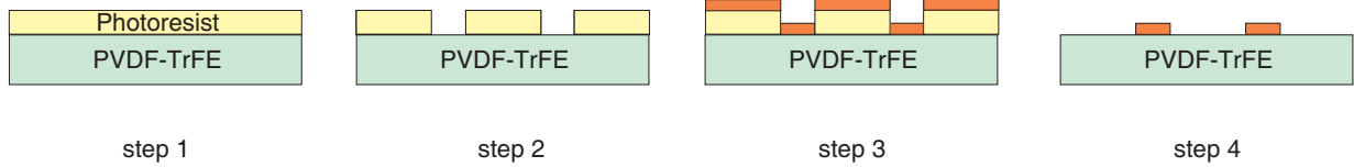
Figure 4.11: Lithography on PVDF films: Spin-coating of the photoresist (step 1), exposure and development process (step 2), metal-electrode deposition (step 3) and lift-off (step 4).
