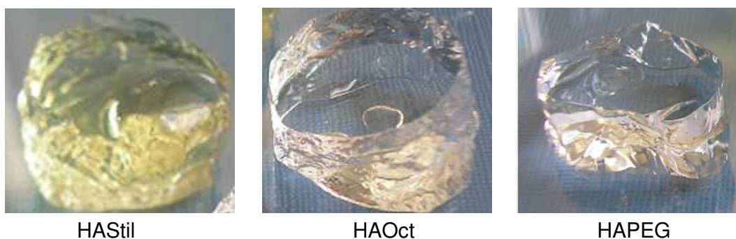
Figure 5.2 Picture of Hyaluronic acid-based hydrogels synthesized by the use of three different type of crosslinkers.
