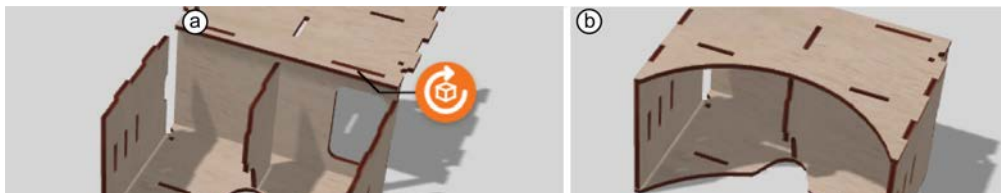
Figure 109: (a) To override a suggestion, the user uses the floating menu item. Assembler 3 presents another orientation of the plate. (b) In this case assembler 3 flips the plate, which leaves the user satisfied with the result.
