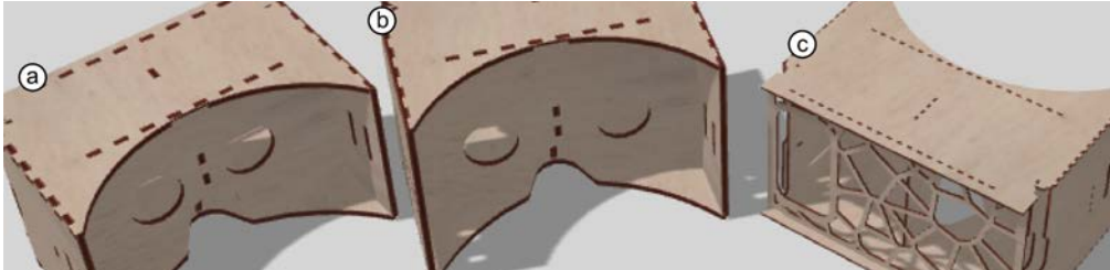
Figure 110: When users have converted the VR headset model to 3D once, the 3D model allows leveraging existing tools (such as kyub [14]) to perform any number of modifications efficiently, such as (a) adjusting the inter-ocular distance, (b) making the headset fit a wider phone by stretching it vertically, (c) or making the headset more comfortable to wear by reducing the weight of the device by decreasing material thickness and removing unnecessary material.
