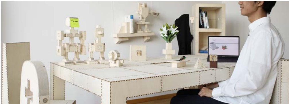
Figure 51: A selection of objects created using kyub, a software system that allows users to design 3D objects for laser cutting. By affording closed box structures, objects made using kyub are very strong. This allows users to make tables, shelves, and chairs that can hold a person. (All shown objects are assembled from 4mm plywood sheets—pressure fit, not glued).
