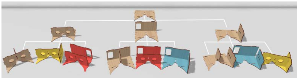
Figure 127: autoAssembler encounters a candidate model more than once (the colored candidates), autoAssembler drops the redundant states (Memoization), by hashing visited candidates. (Here shown with three candidates each for visual clarity).
