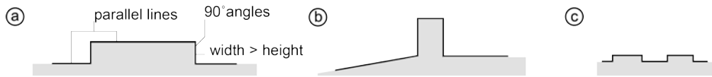
Figure 112: (a) The ideal finger joint has 90-degree angles, a top line parallel to the edge and has a bigger width than height (b) this finger joint has a much lower probability, it could just as well be some aesthetic feature of the model? (c) repetitions of a pattern increase its probability.
