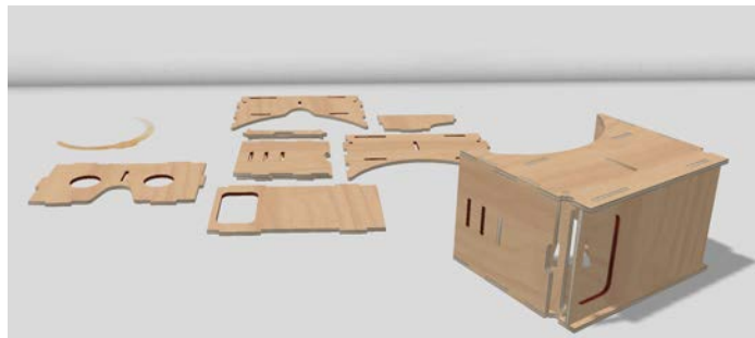
Figure 7: We reconstruct 2D cutting plans into 3D models as shown here at the example of a VR headset represented as 2D plates and the resulting 3D assembled model. We built an automatic pipeline to achieve this, and we provide an interactive fallback for models that turn out to be challenging.
