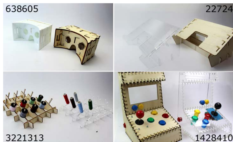
Figure 20: Four of the models we converted and fabricated as part of the first technical evaluation. (thingiverse IDs on the label)
