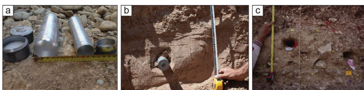
Figure 3.7 Illustration of the two sampling techniques used for IRSL dating. (a) Sampling tools: aluminum tubes and lids for hammering. (b) Sampling with aluminum tubes during the day. (c) Sampling locations after sampling at night into conductive bags.
