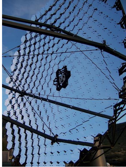
Figure 4.3: The 350 hexagonal mirrors on VERITAS reflector of one telescope.
