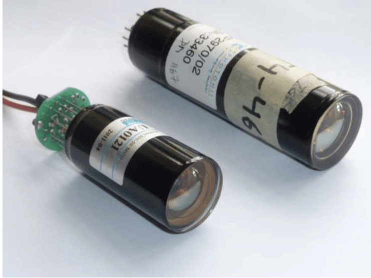
Figure 4.5: Photograph of the Photonis XP2970 PMT (right), replaced with the Hamamatsu R1056010020 (left) in 2012 [118].
