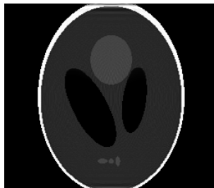
Figure 2.4: Reconstruction of the three-dimensional phantom, which lay partially within the field of view, with the modified version of DIRECTT.
