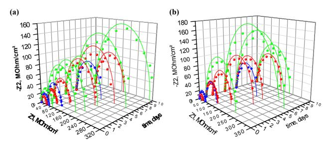
**Figure 45.** Nyquist Plots of coatings containing 10 wt-% (left) and 20 wt-% (right) containers without (red) and with (green) hydroxyquinoline. Blue curves represent the blank coating. Points represent measured and continuous lines modelled impedances.
