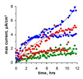
**Figure 47.** Maximum current densities obtained by SVET measurements for scratched alkyd coatings on aluminium in 0.1 M NaCl solution. Blue: blank coating (no containers), red: coating with 10 wt-% containers, green: coating with 20 wt-% containers. Lines are drawn to guide the eye.
