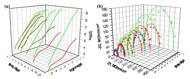
**Figure 44. (a)** Comparison of the impedance of a coating with defects (red) and a homogeneous defect-free coating (green) with both 10 wt-% containers in the Bode Plot. (b) Nyquist Plot of a coating containing 5 wt-% containers without (red) and with (green) hydroxyquinoline. Blue curves represent the blank coating. Points represent measured and continuous lines modelled impedances.
