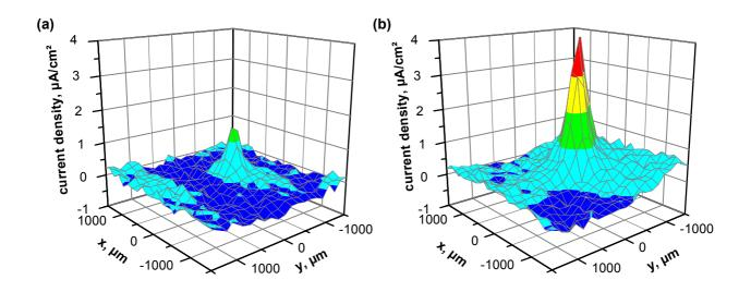
**Figure 7.** Graphical representation of the current density distribution measured 300µm above a scratched polymer-film on an aluminium substrate in a 0.1 M NaCl solution. (a) after 30 min and (b) after 8 hrs.
