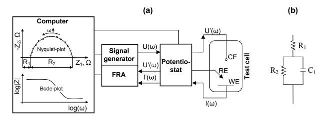
Scheme 4. (a) Impedance setup using a frequency response analyzer (FRA). CE calomel electrode, RE reference electrode, WE working electrode. (b) electrical circuit of a resistor ( $R_1$ ) in a series with a parallel circuit of another resistor ( $R_2$ ) and a capacitor ( $C_1$ ).
