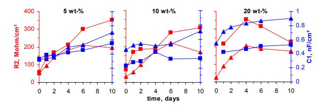
**Figure 46.** Ohmic resistance (R<sub>2</sub>) and capacitance (C<sub>1</sub>) of an alkyd polymer-film with different mass fractions of silica-PS capsules on aluminium with ( $\blacksquare$ ,  $\blacksquare$ ) and without ( $\blacktriangle$ ,  $\blacktriangle$ ) 8HQ in the capsules, obtained from the short circuit analysis (R<sub>1</sub>(R<sub>2</sub>/C<sub>1</sub>)-circuit) of the impedance spectra shown in Figure 44(b) and Figure 45
