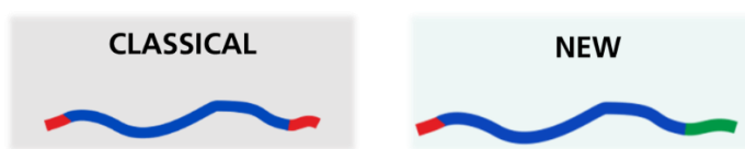
Figure 2.1: Classical vs. new structure of amphiphilic block copolymer; red = permanently hydrophobic block, blue = hydrophilic block, green = thermoresponsive block.
