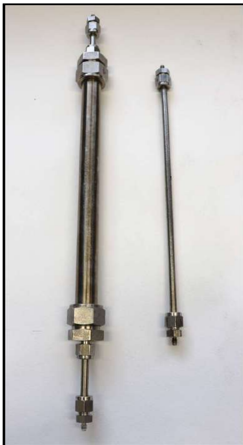
Figure B3. The used stainless steel tubular reactors: Left) the prototype scale reactor , with inner diameter 21 mm, outer diameter 25mm and length 280 mm. Right) reactor with inner diameter of 4.6 mm, outer diameter of 6.5 mm and length of 250 mm.
