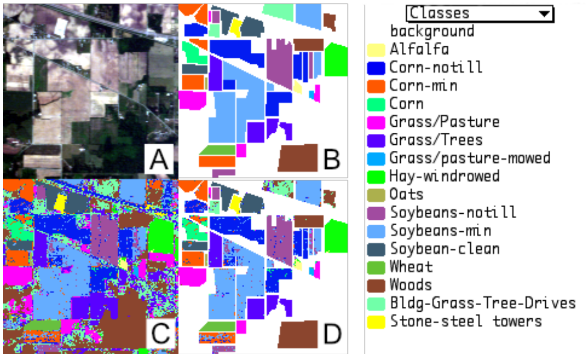
Figure 39: A; The hyperspectral training image cut out from the original image to the dimensions of the ground truth ROIs true color image of the scene (Red: band 27 (646.7 nm), Green band 17 (547.6 nm), Blue band 7 (449.1 nm). B; The Indian pines ground truth with classes in the original color-scheme, [6]. C: DeepGeoMap 165 epoch model classification of the Indian Pines scene with an overall accuracy of 96.21%. D: DeepGeoMap 165 epoch validation image classification showing the misclassifications in each validation ROI. The VA is 96.04%.
