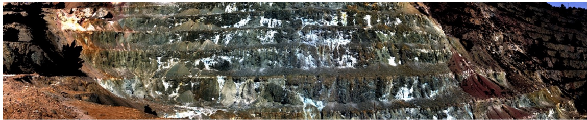
Figure 19: "NDVI & shadow masked reflectance field scan. Vegetation and areas of shadow (high SNR) are masked out and shown in black. (RGB composition: R: band 63, G: band 38, B: band 13.)", Koerting (2021) [24].
