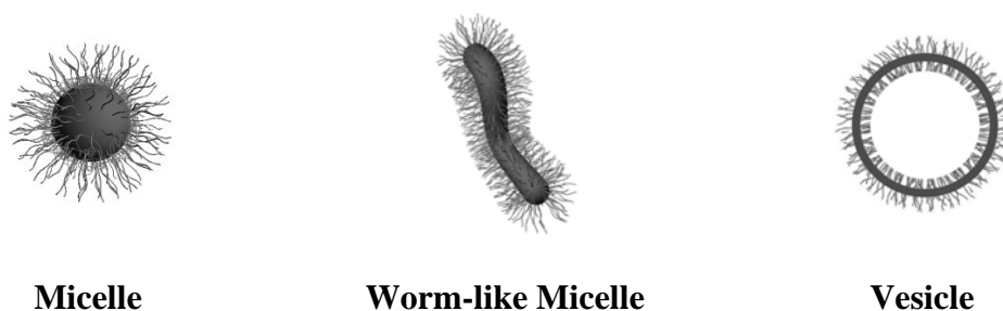
Figure 2.6. Possible morphologies of block copolymer aggregates occurring in dilute solutions.
