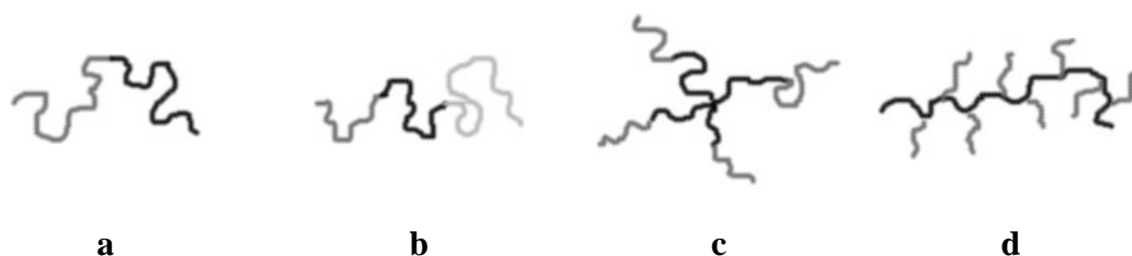
Figure 2.1. Various architectures of block copolymers: a) diblock copolymer, b) triblock copolymer, c) star, d) brush.
