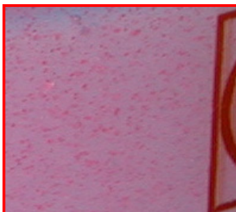
Figure 27. The formation of the coagulum during the ab-initio emulsion polymerization of styrene initiated with PEGA 200 in the presence of PhEDB
