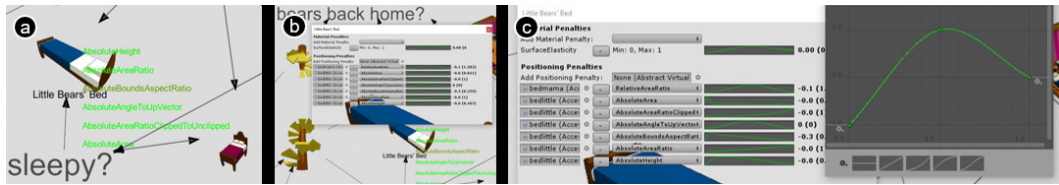
Figure 8: (a) By hovering over ‘little bear’s bed’ we preview its parametric description. (b) This popup window details all parameters and current fitness values for ‘little bear’s bed’. (c) We change the valuation for ‘surface elasticity’ to get a somewhat soft ‘bed’. The 13 virtual objects in Goldilocks have a total of 91 rules.
