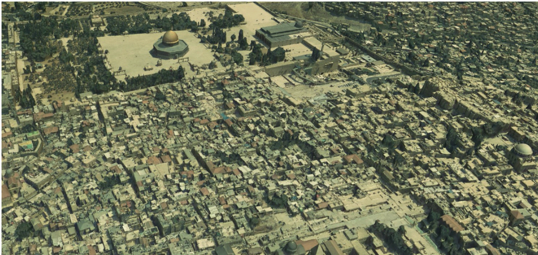
Figure 2: Section of a point cloud of the Old City of Jerusalem in true colour. In total, the invariant mass data set comprises almost 20 billion points, with a storage requirement of almost 500 GB, a point spacing between 0.511-0.023 cm and an average horizontal point density of 119 pts/sqm.
