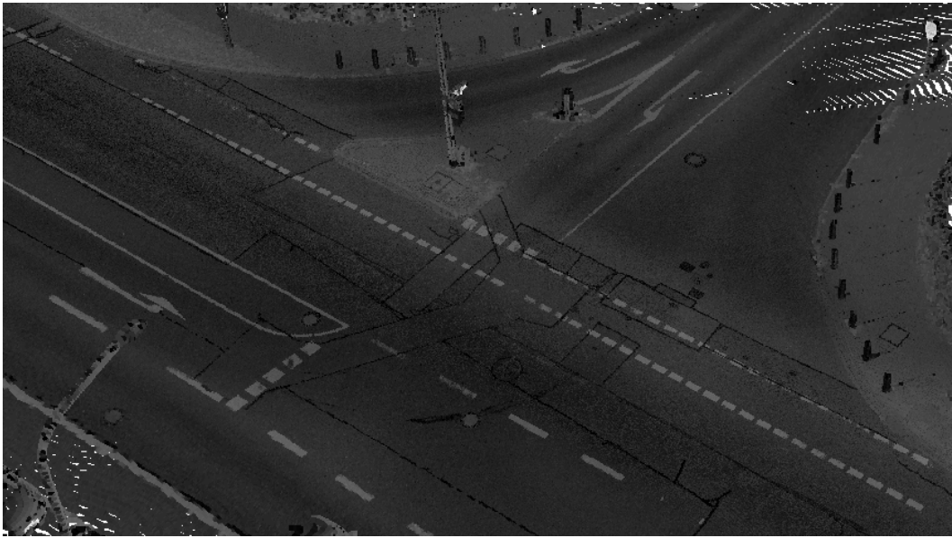
Figure 2: 3D point cloud of a crossing with road markings. Intensity values are represented in grayscale, lighter colors have higher intensity values.
