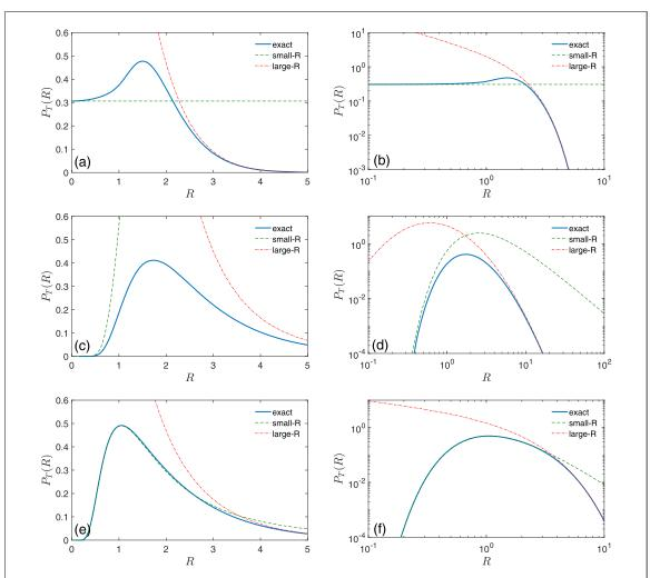
**Figure 4.** Probability density function  $P_T(R)$  of the range and its small-R and large-R asymptotic behaviours, for model I (a) and (b), model II (c) and (d), and model III (e) and (f), plotted on linear (a), (c), (e) and log-log (b), (d) and (f) scales. We set  $D_0 = 1$ , T = 1, a = 1, and  $D_B = 1$ . Compare this behaviour to the Brownian limit in figure 1.
