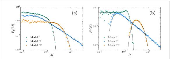
**Figure 5.** Comparison of the probability density functions  $P_T(M)$  (a) and  $P_T(R)$  (b) for the three random diffusivity models. Solid lines show the analytical formulas whereas symbols represent the empirically renormalised histograms obtained from Monte Carlo simulations with  $10^4$  runs (time step  $10^{-2}$ ). We set  $D_0 = 1$ , T = 100, T = 1
