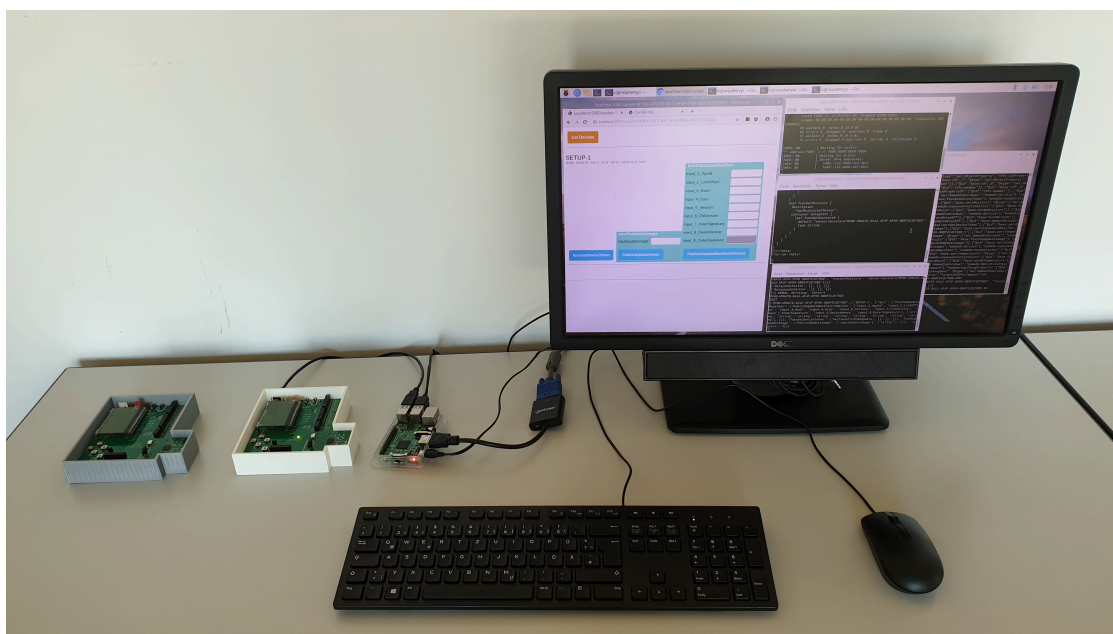
Figure 4. Testbed with a Raspberry Pi 3B and a CC2538dk Development Kit consisting of two CC2538EM microcontrollers plugged into the SmartRF06 Evaluation Boards and used as a 6LoWPAN Border Router and an IoT device (wireless and battery-powered) on the left.
