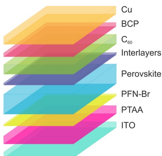
Figure 3.3: Exemplified layer stack of a typical perovskite solar cell studied in this work.
