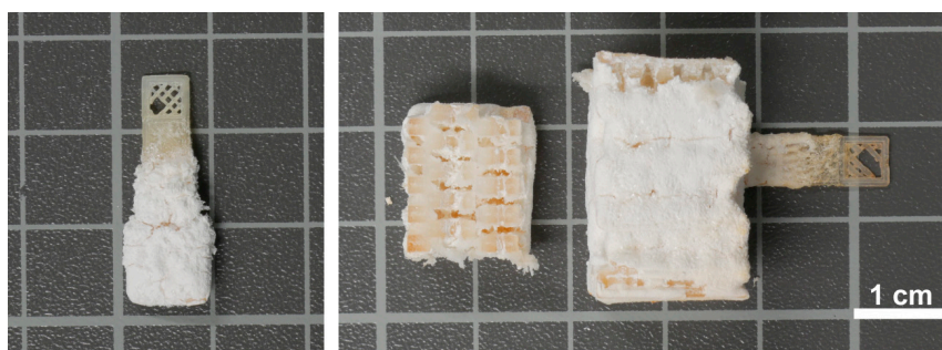
Figure 5. Mineral-coated samples: scaffold type P2 (sample G03 (left)) and scaffold type P3 (sample G07 (center and right)). Sample shown in the center is cut open to show the inner section of the scaffold. The scale bar applies to all images.
