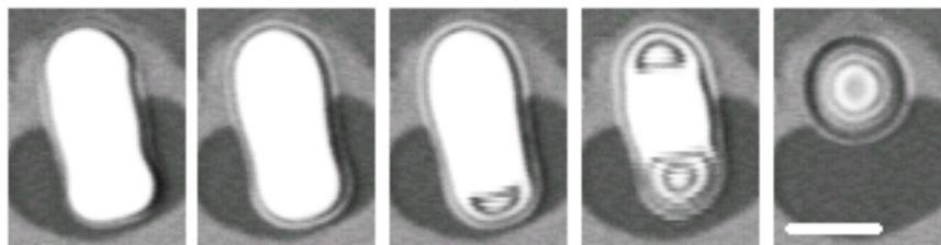
Figure 7.4. Sequence of optical microscopy images showing the melting of a \approx 240 nm thick \text{C}_{24} terrace ( 10\mu\text{m} scale bar). In the first three images, the liquid stripe wetting the stepped perimeter (white contour) widens and then two distorted drops form in the regions of highest in-plane curvature. Finally the entire structure is molten.
