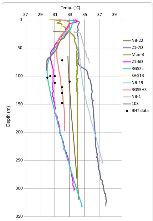
**Fig. 4** Continuous T-logs measured with a conventional temperature probe in seven wells during this study. Additionally three continuous T-logs (NB-1; NB-19; NB-22) and bottom-hole temperatures (BHT), provided by the MRMWR, measured in a cluster of nine wells close to the Al Khawd dam (for location see Figs. 1, 2)
