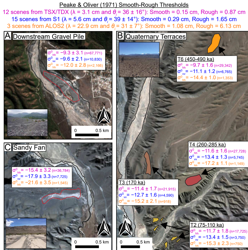
Figure 5.4 – Differences in X-, C-, and L-band \sigma^0 (mean \pm standard deviation in dB) from three endmembers. The locations are indicated in Figure 5.5A. (A) shows a large man-made gravel pile associated with in-channel gravel extraction, (B) shows the Quaternary terraces with dates from Tofelde et al. (2017), and (C) shows a sandy outwash fan associated with a small debris-flow prone sub-catchment. The color scheme (pink for TSX/TDX, blue for S1, and orange for ALOS2) is used consistently in the chapter and Appendix C. Note the Peake and Oliver (1971) smooth-rough thresholds listed above the figure. The river (black outline) always flows approximately north to south. Inset pictures taken from each area during fieldwork. Basemap imagery is the S2 scene used in Figure 5.3.
