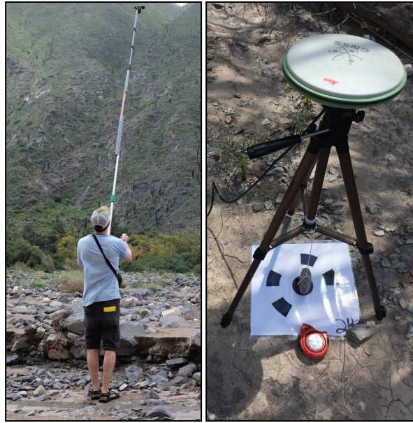
Figure 4.7 – Sony \alpha 6000 24 megapixel camera affixed to mast for photo collection at a height of 4.5–5 m (left) and differential GPS measurement of coded targets (right).
