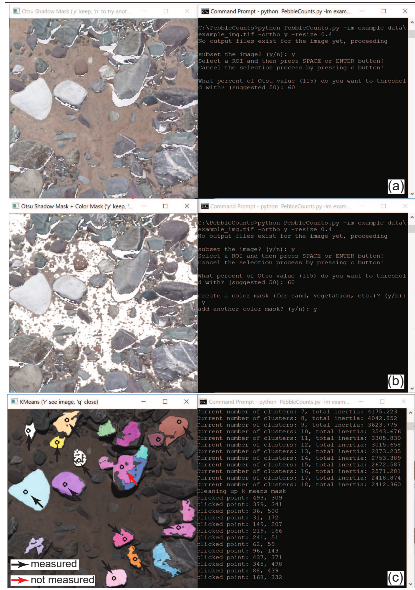
Figure B2 – Example of command-line and pop-up interface for PebbleCounts . (a) Interactive Otsu thresholding using percentage of Otsu value and yes ('y') or no ('n') confirmation. (b) Interactive color masking by yes ('y') or no ('n') and resulting color mask after selection. (c) K-means clustering and pop-up window for pebble selection by left clicking, with black arrows measured in final output and red arrows ignored after right-click removal (see Fig. B3).
