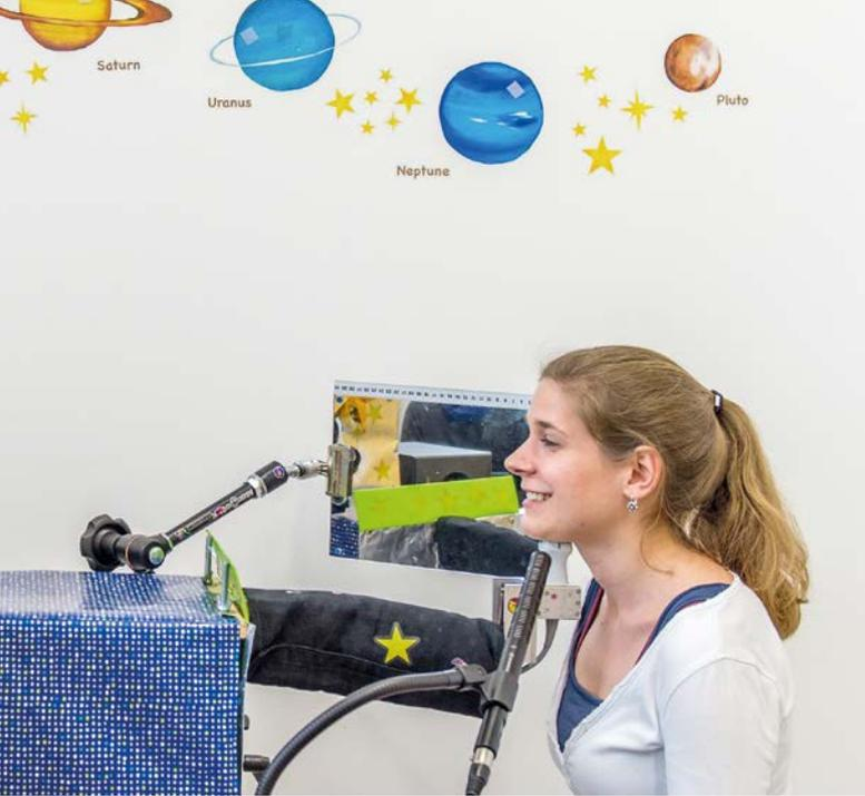
*The ultrasound probe is the centerpiece of the experimental design.*
