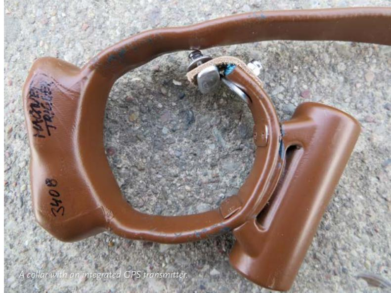
A collar with an integrated GPS transmitter.
