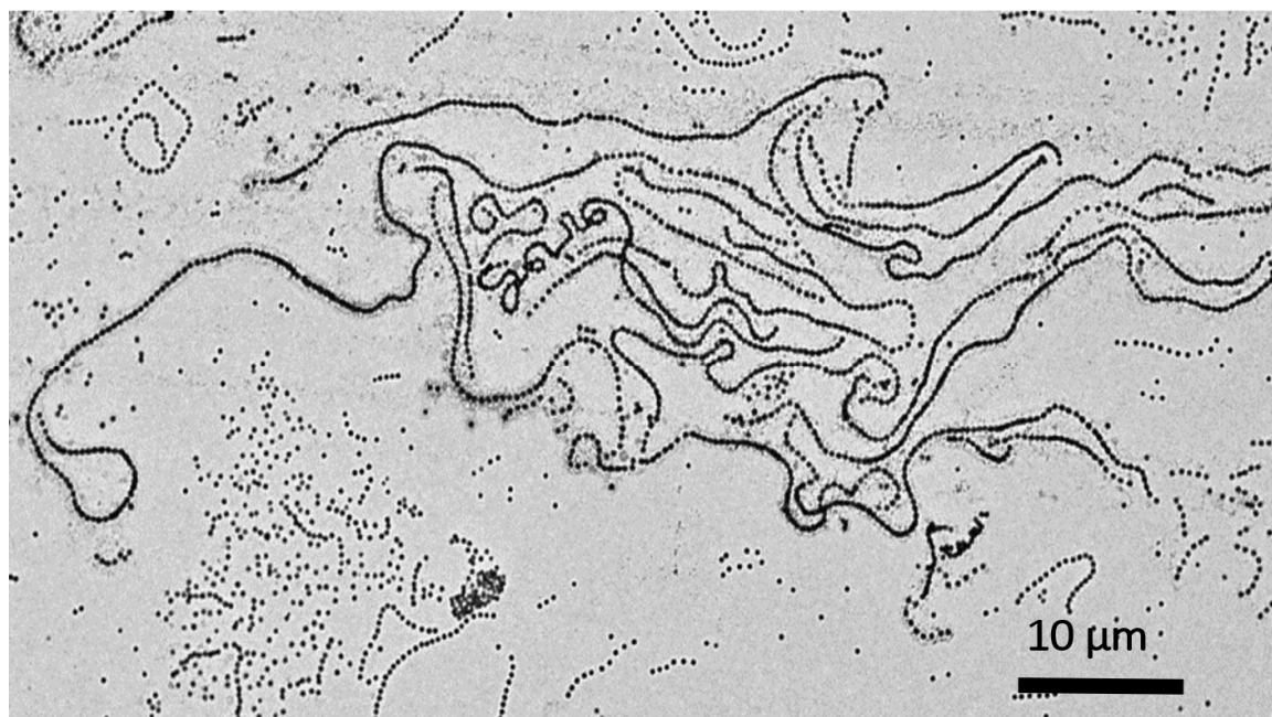
Figure 50: Various TEM images that show long microgel strands. 141
