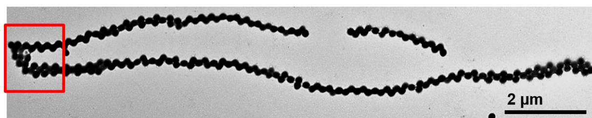
Figure 89: TEM image of a cross-linked microgel strand where on the left side (red) the L-shaped structure can be seen.
