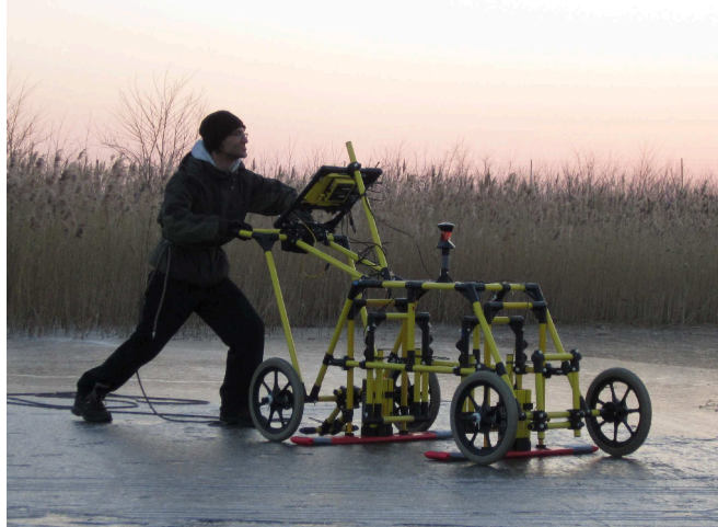
Figure 1.1: A common offset (CO) GPR, with red antennae under the cart, digital video logger with screen in front of the operator and prism for position tracking mounted on top of the cart (standard measurements for bathymetric mapping and sedimentation rate estimation on a frozen lake).
