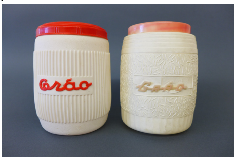
Figure 2. Example of two plastic recipients with red caps made of PS (left) and PE (right) showing different colour stabilities. In both caps PR 53 was identified as the red colouring agent.
