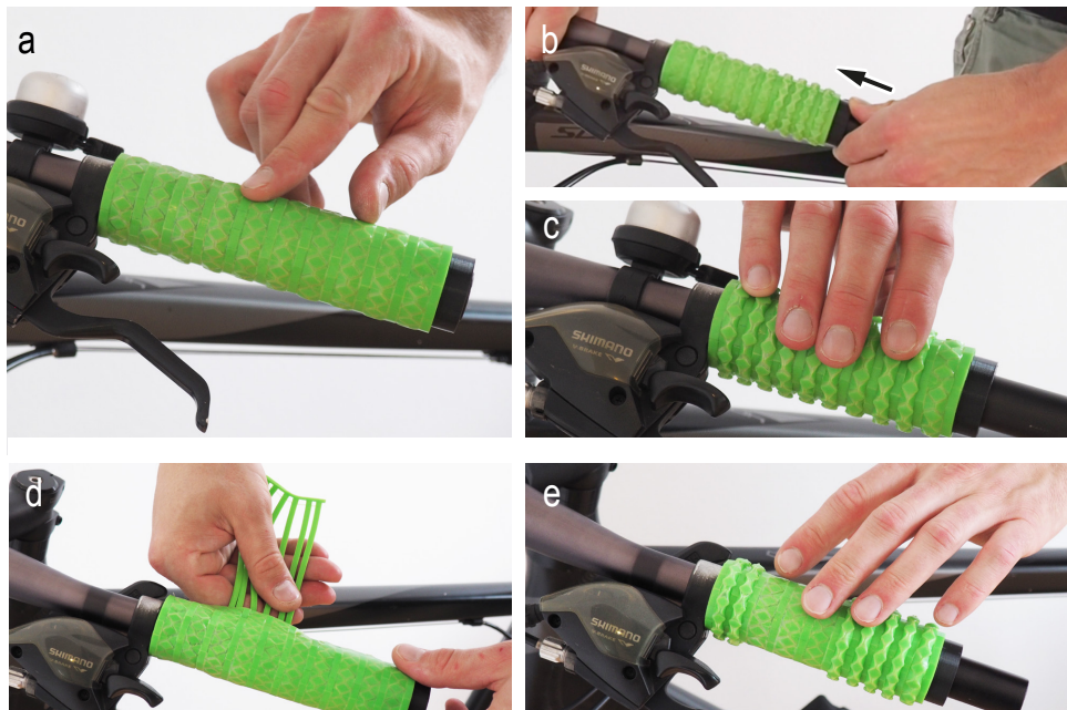
Figure 6.6: (a) Designers fabricate one single bicycle grip that they (b) actuate continuously to different levels, (c) to feel the tactile qualities during rapid prototyping. (d) By inserting spacers after fabrication that (e) deactivates selected rows allows them to further investigate the grip’s ergonomics.
