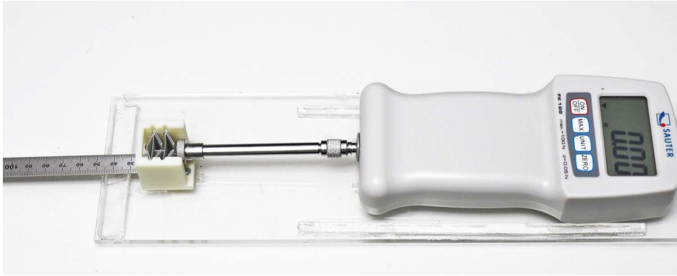
Figure 5.24: We measure the forces using a force gauge (error 0.05 N), and the stroke length using a ruler (error 0.5 mm).
