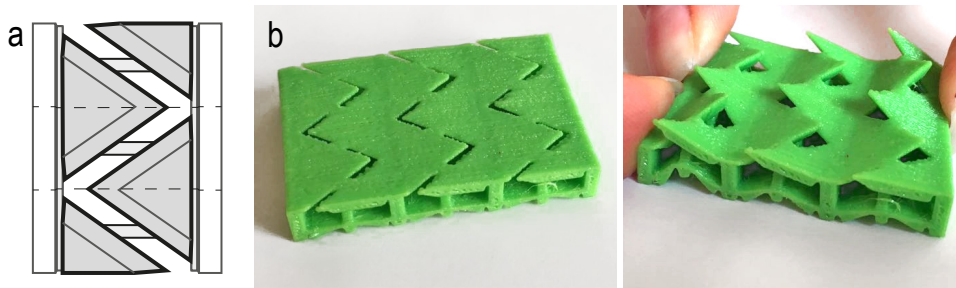
Figure 6.14: (a) Leaving gaps between the members of the cell top (b) allows for creating spiky textures.
