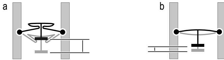
Figure 5.22: (a) The spring we use in our bit cells is longer and thus weaker than (b) conventional bistable springs. Or, for the same force, our cells produce more stroke length.
