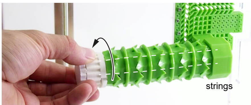
Figure 6.4: Users transition through the door handle’s embedded textures by turning the knob. That winds up the strings on the inside, which compresses all cells and forms the textures.
