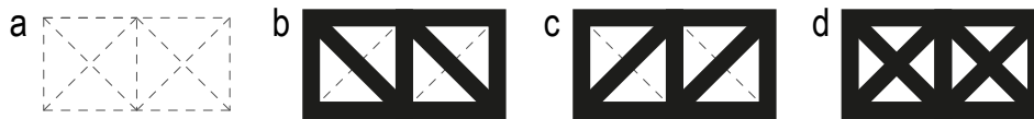
Figure 3.3: (a) The basic grid structure allows reinforcing rigid member cells (b-c) with one diagonal or (d) two diagonals.
