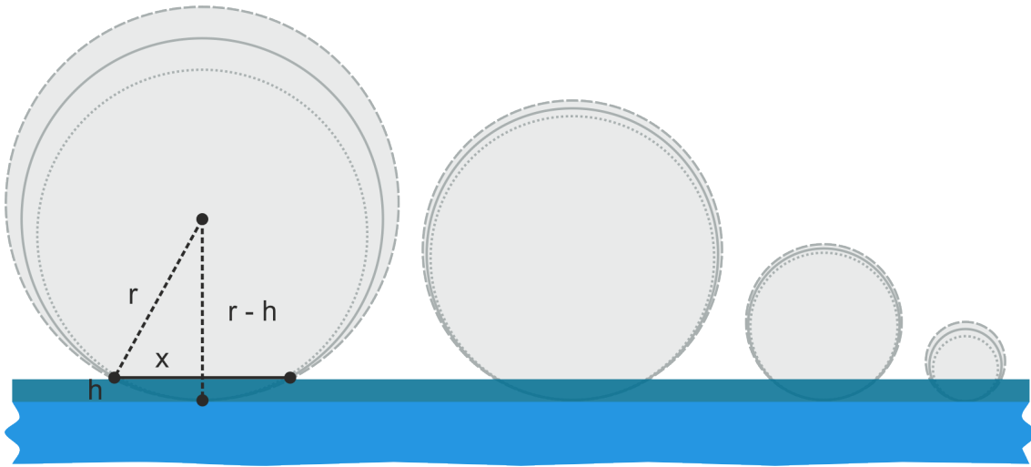
Figure 5.1 Schematic illustration of the influence of particle size distribution on the patch diameter. Four particle sizes (solid line) used in this research, (5.06 \pm 0.44) \mu\text{m} , (4.08 \pm 0.11) \mu\text{m} , (2.12 \pm 0.06) \mu\text{m} and (1.01 \pm 0.10) \mu\text{m} , are depicted inside a thick ink film, with upper (striped line) and lower (dotted line) size distribution limit. Given variables are particle radius r , ink film thickness h and half patch diameter x .
