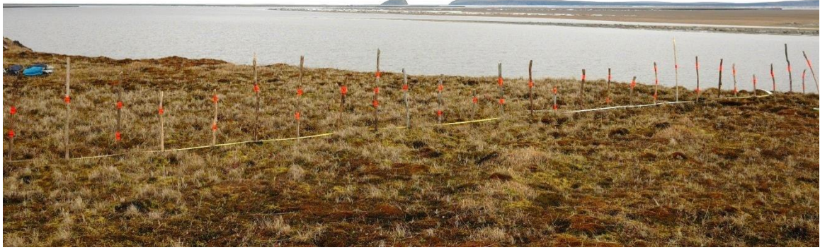
Figure 2-5: In-situ monitoring of cliff-top erosion on Kurungnakh Island. The field photo from 21st of June 2015 shows the field of view of the time lapse camera on the eroding cliff top. The camera monitored a 15 m long transect that was set up perpendicular to the cliff-top line and consisted of 29 equally spaced (50 cm apart) wooden stakes. Photo: Samuel Stettner, June 2015.
