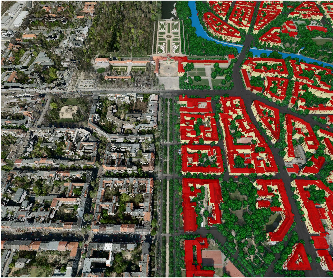
Figure 5.10: Examples of a 3D point cloud rendered with different point-based rendering techniques taking into account object-class information per point. (left) All points are rendered as point splats with color information from aerial images. (right) Buildings are rendered with solid rendering, vegetation with point spheres, and ground with point splats. The color depends on the surface category.
