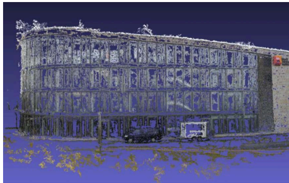
(f) Dense image matching point cloud generated with Autodesk's 123D Catch (Autodesk 2017).
