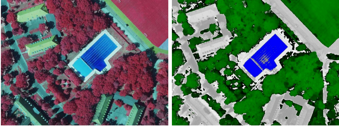
(a) Point cloud with color information from an aerial true orthophoto with CIR information. Red colors indicate near infrared, which are beyond the wavelengths for the color red. (b) Point cloud with colors based on NDVI information from CIR images (green - vegetation; blue - water; gray - areas without vegetation).
