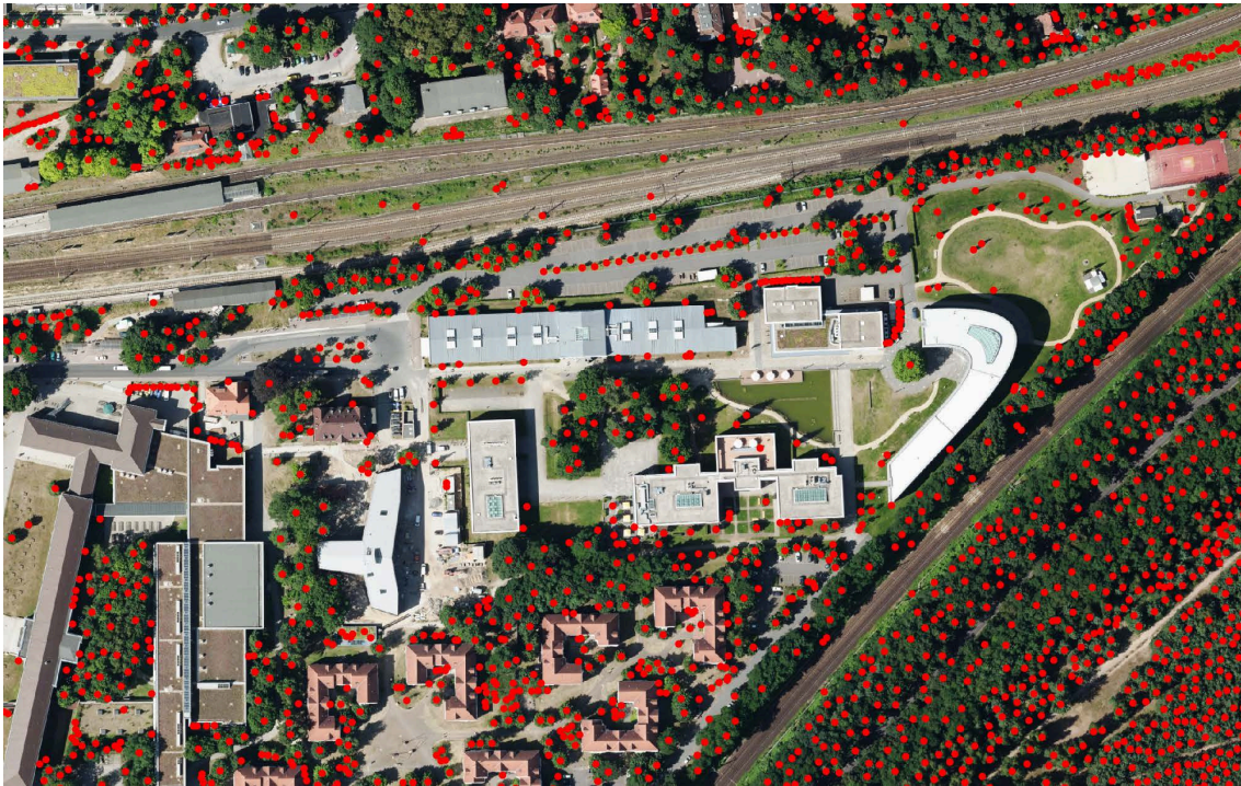
(a) 2D illustration of tree cadastre. Tree positions are illustrated as red circles over the aerial image.
