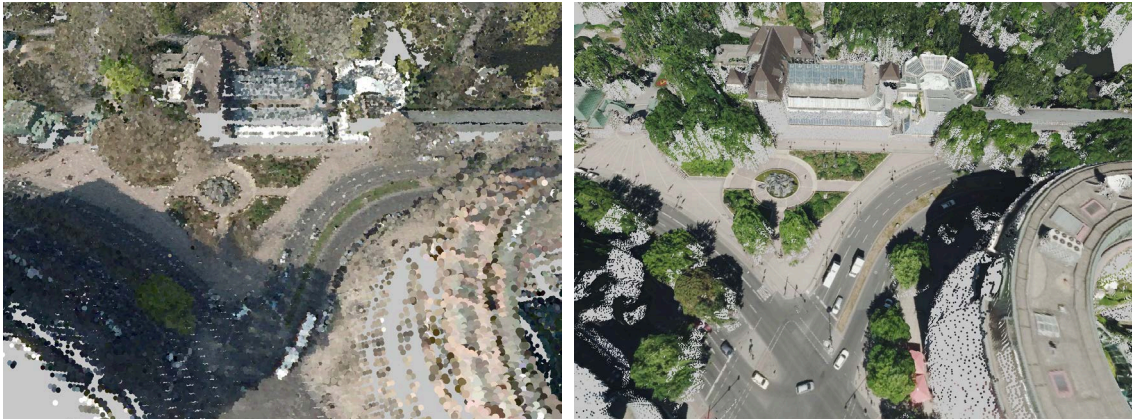
(a) LiDAR scan of Berlin with colors from aerial images. (b) Dense image matching scan of Berlin with colors from aerial images.
