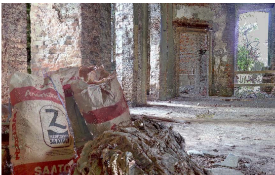
(g) Indoor scan of a building captured with a terrestrial LiDAR scanner.
