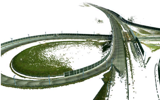
(c) Mobile mapping point cloud captured with a LiDAR scanner mounted on a vehicle.
