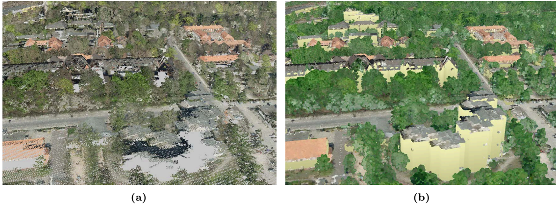
Figure 5.7: (a) Example of a massive 3D point cloud rendered in a uniform way by GL_POINTS primitives and textured by aerial photography. (b) Same scene rendered by class-specific point-based techniques: different object classes can be better distinguished, holes on façades are filled, and visual clutter in the background is reduced.
