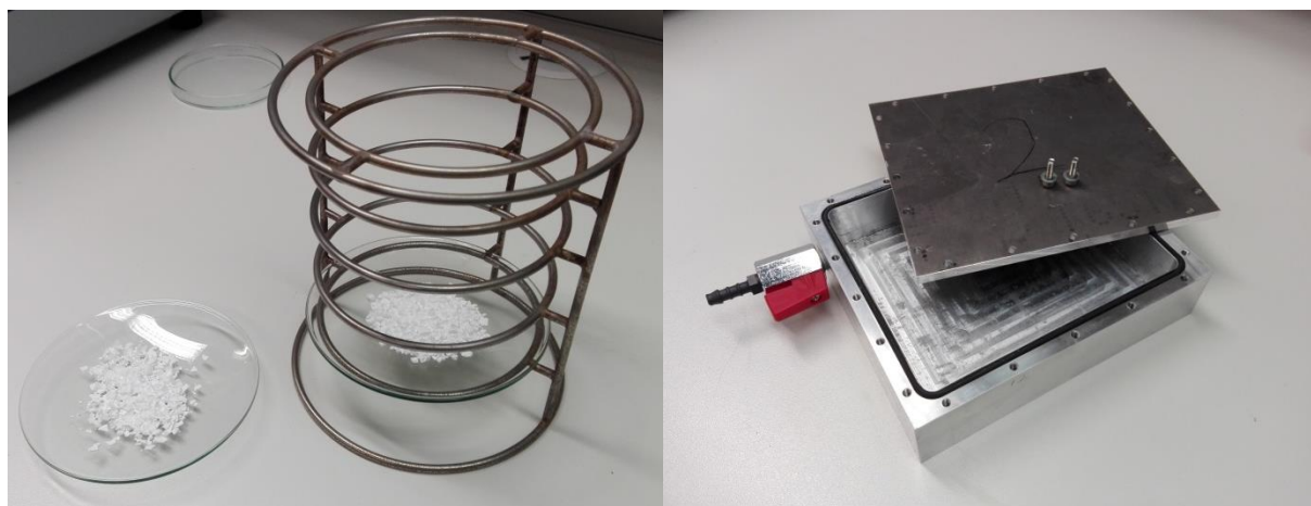
Figure 3.1: Left) Sample drying rack, holds six samples for drying in a desiccator. Each sample is placed on a 13 cm wide watch glass. The whole rack fits into a desiccator. Right) travel desiccator for amorphous samples, holds 10 sample vials at a time each containing ~5 grams of sample.
