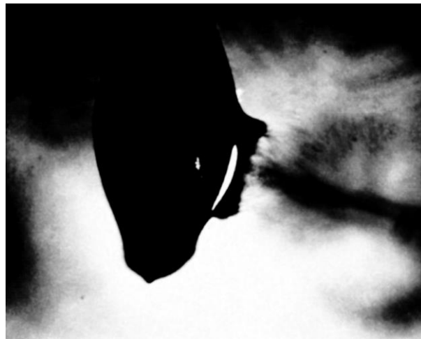
Figure 32: Shadowgraphy images of the dispersion plume for an ACN/H 2 O 1:1 mixture at 8 \mu\text{s} after the beginning of phase explosion
