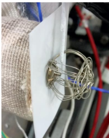
Figure 17: Spherical repeller electrode at the end of the ion transfer tube. The sample capillary tip is just before that of the ion transfer tube. A Teflon sheet insulates the heating element from the high voltage components
