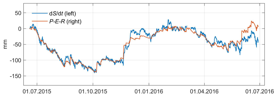
Figure 10. Time series of water storage at Wettzell (as a deviation from the initial storage value at the beginning of the study period, arbitrarily set to 0), with the measured iGrav006 gravity-based storage time series (blue line) (left side of Eq. 3) and the optimized storage time series (red line) after optimization following the right side of the water balance equation (Eq. 3).
