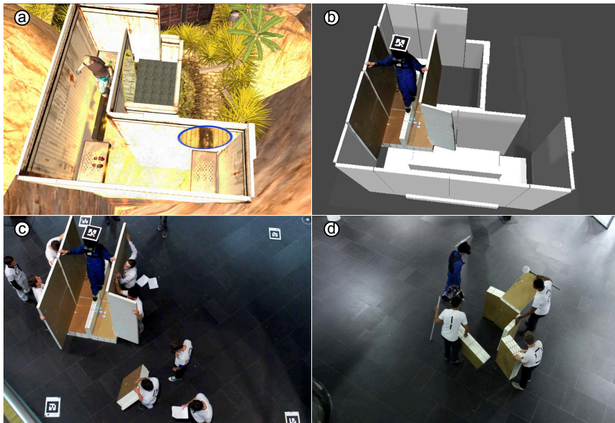
Figure 25: TurkDeck is a prop-based virtual reality system that let's users not only (a) see and hear a virtual world, but also (b) feel it. Conceptually, the user is in a fully populated physical world. (c) In reality, however, TurkDeck's physical room is almost empty. "Human actuators" present and operate props only when and where the user can actually reach them. (d) By reusing generic props, TurkDeck minimizes the required props to what human actuators can carry, still allows producing virtual worlds of arbitrary size.
