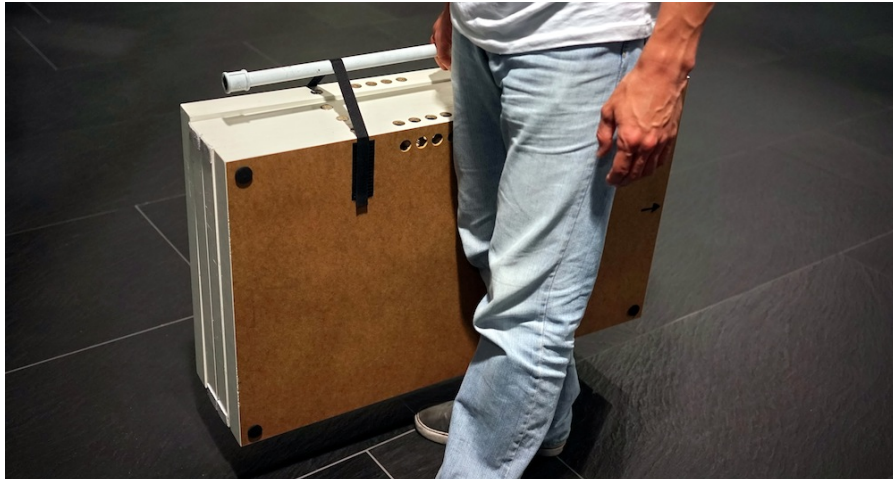
Figure 30: The foldable board and the stick pack into a 90x55x20cm package that human actuators can carry like a suitcase.
