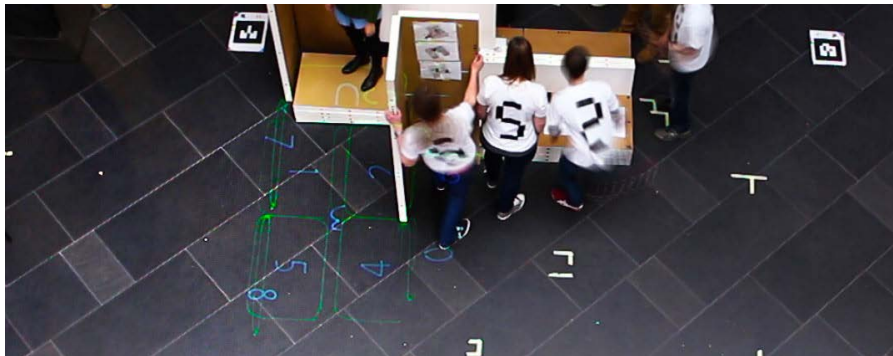
Figure 33: The projected human actuator interface consists of green board outlines and blue human actuator IDs.
