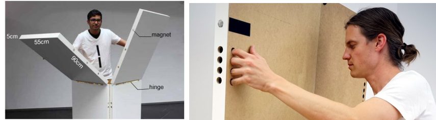
Figure 28: The board folds in four. Joints and magnet connectors help human actuators reconfigure the boards. Finger holes enable actuators to lift boards easily.
