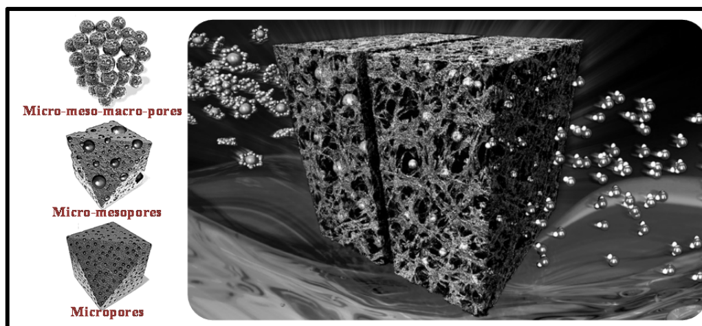
Figure 6: Depiction for the different porosity and its importance in mass transfer.
