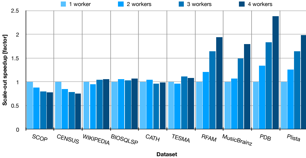
Figure 2.12: Speed up of SINDY when using four instead of only one worker, while maintaining a parallelism of 10.
