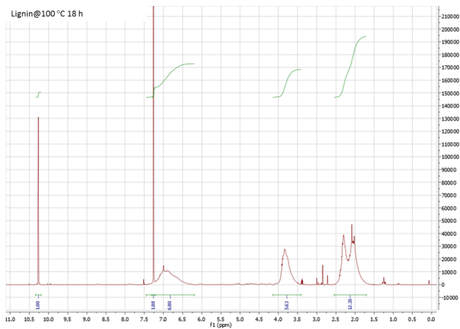
Figure C-11 1 H NMR spectrum of heat-treated lignin at 100 °C 18 h in CDCl 3 solvent after acetylation (2,3,4,5,6-pentafluorobenzaldehyde as an internal standard, 10.26 ppm).
