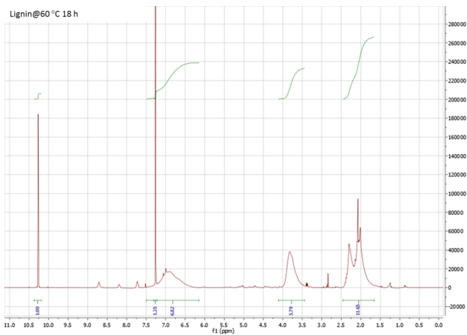
Figure C-9 ^1\text{H} NMR spectrum of heat-treated lignin at 60 °C 18 h in \text{CDCl}_3 solvent after acetylation (2,3,4,5,6-pentafluorobenzaldehydes as an internal standard, 10.26 ppm).
