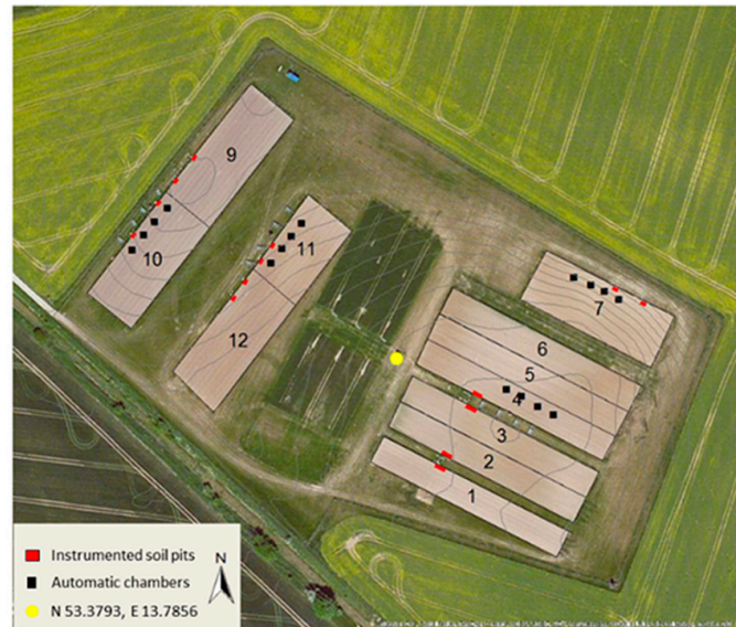
Figure 1. The CarboZALF experimental area near Dedelow (NE Germany): plot design and instrumentation.
