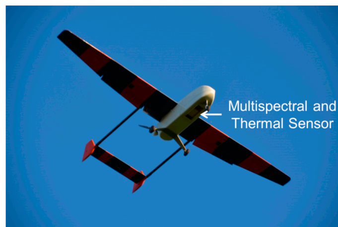
Figure 2. The Carolo P360 unmanned aerial vehicle (UAV) during a mission with open landing gear doors.
