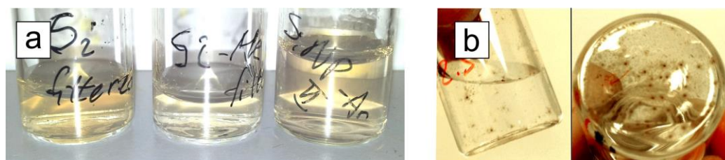
Figure 5.7. (a) The color of three silicon nanoparticle aqueous suspensions prepared by laser ablation (from left to right) without gas (SiNP), with He (SiNP He), and with Ar blowdown (SiNP Ar II). (b) Precipitated UV-exposed silicon nanoparticles SiNP Ar decorated with azobenzene surfactant.
