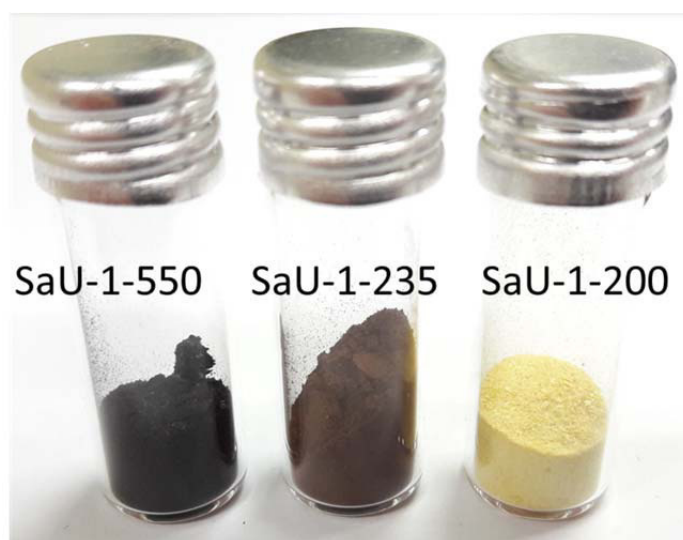
Figure SI-4.2.10. Photographs of the SaU-1 crystals after thermal condensation for 2h at 200 °C (sample SaU-1-200, right), 235 °C (sample SaU-1-235, middle) and 550 °C (sample SaU-1-550, left).
