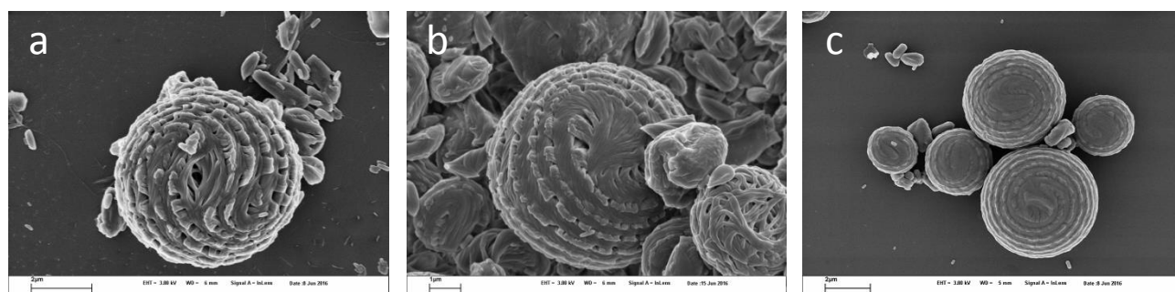
Figure VI.10 Particles resulting from polypeptide-toluene in water emulsions of (a and b) \text{PBDG}_{155} , and (c) \text{PBLG}_{159} . Scale bars = (a and c) 2 \mu\text{m} , (b) 1 \mu\text{m} .
