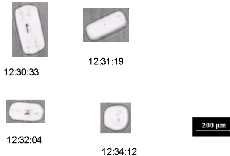
Figure 6.6: Images of the four single ice crystals detected by the CPI in the thin cloud at about 3 km altitude. Provided by Jean - François Gayet.
