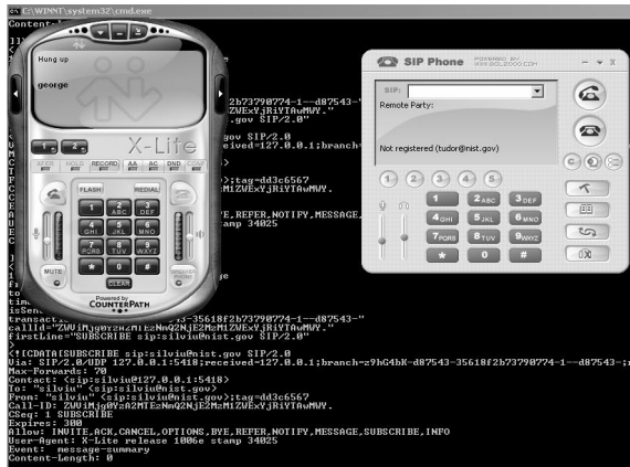
Figure 8: Simple mode of using the IN Helpdesk using SIP phones. The Mobicents server is running in the background
