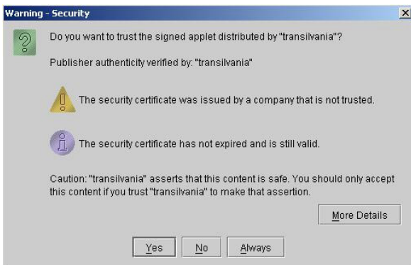
Figure 8: Warning of loading a signed applet, which requires additional privileges for the execution of commands outside the sandbox
