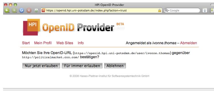
Figure 3: The HPI OpenID Provider requests authorization from the user to share identity information.
