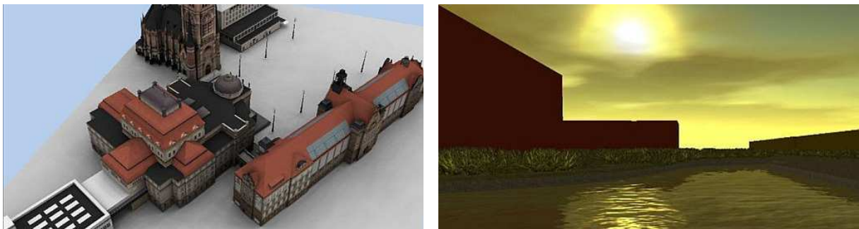
Figure 4: Examples for rendering styles and effects relevant for 3DGeoVE: ambient occlusion simulating daylight (left) and sun, clouds, atmospheric effects, and water shading (right).
