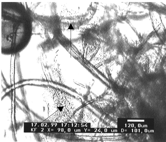
Figure 171. Optical photograph (x100) of used cellulose fibres with precipitated MCCbB gel-like dispersion prepared in a bath containing 20 wt% casein. ↓ shows the coated cellulose fibres by MCCbB
