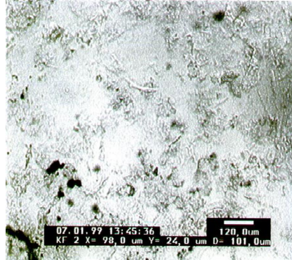
Figure 103. Optical microscope microphotographs of MCChB gel-like dispersion prepared in coagulation bath containing 20 wt% casein (x100)
