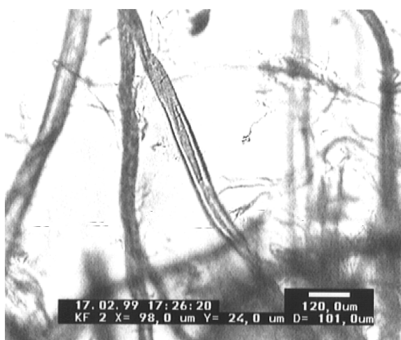
Figure 169. Optical photograph (x100) of used cellulose fibres
