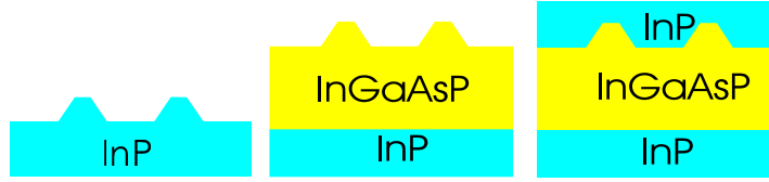
Figure 6.1: Sketch of the geometries of the three samples investigated in this Chapter: a simple, strain-free grating at the surface of an InP substrate (left), a strained-layer surface grating (center), and a similar grating, additionally buried under an InP layer (right).
