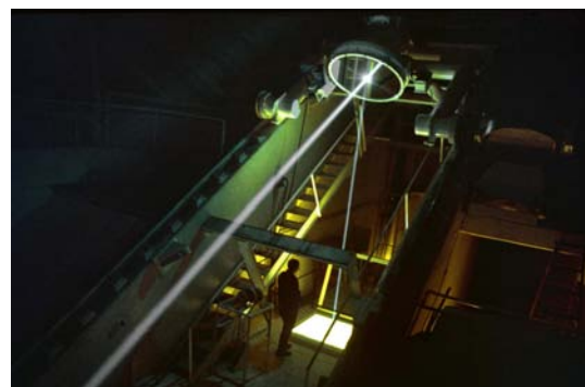
Figure 4.1.: Left. The McMath–Pierce telescope at Kitt Peak, Arizona, where most of the observations were done. In the background the NSO vacuum telescope, which now hosts the SOLIS instrument. Right. Lightpath in the tunnel of the McMath–Pierce telescope. The star- (or sun-) light is reflected by the ceolostat (mirror 1) at the top of the building into the tunnel. At the bottom of the tunnel (buried into the ground) the light is reflected back up to mirror 3 (the one shown in the picture), which can be adjusted to reflect the light to the appropriate instrument. Images courtesy of NOAO/AURA/NSF.
