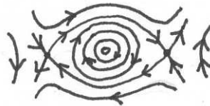
FIG. 7: Organization of phase space for an integrable system, corresponding to the phase-space picture of a frictionless pendulum. The picture shows one elliptic point surrounded by separatrices associated with the hyperbolic points on the left and right.
