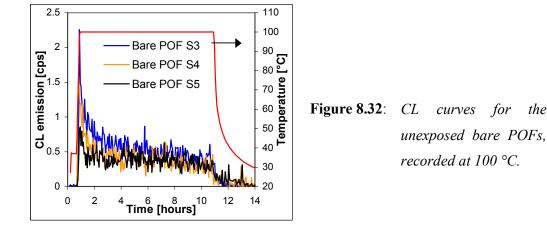
CL emission to the transmission loss that occurs at the early stages of climatic exposure of POFs.
