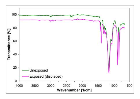
**Figure 8.13**: ATR-FTIR spectra of the unexposed and exposed cladding S1.
