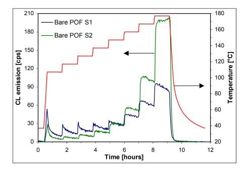
Figure 8.10: CL curves for the exposed bare POFs S1 and S2.
