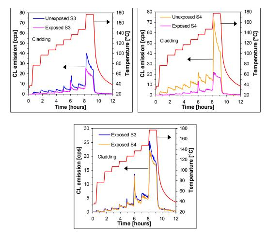
**Figure 8.38**: *CL curves for the unexposed and exposed cladding samples S3 and S4. The exposure condition was 90 °C / low humidity.*
