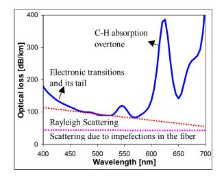
**Figure 4.1**: Schematic spectral representation of optical loss factors in (PMMA) POFs.
