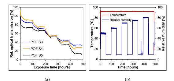
**Figure: 8.39**: (a) Relative optical transmission through bare POFs, measured during the exposure to climates of steady temperature with varying humidity; (b) Applied temperature and humidity scheme recorded during the exposure.
