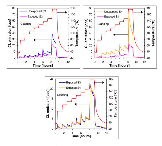
**Figure 8.34**: *CL curves for the unexposed and exposed cladding samples S3 and S4. The exposure condition was 92 °C / 50 %RH*
