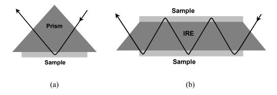
**Figure 7.6**: Schematic representation of attenuated total reflectance in: (a) single reflection prism; (b) multireflection element.
