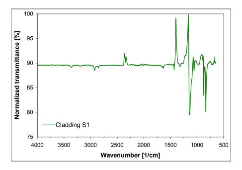
**Figure 8.15**: Difference IR spectrum (ATR-FTIR spectrum of the exposed minus unexposed cladding S1).
