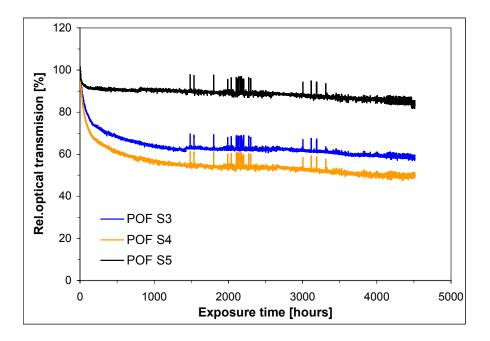
Figure 8.27: Assumed optical transmission function of time through (averaged over three wavelengths) bare POFs S3, S4 and S5 under the exposure climate 100 °C / low humidity after the subtraction of the linear loss from 100 %.
