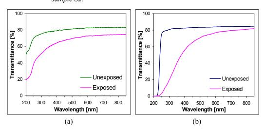
**Figure 8.19**: UV/visible transmittance spectra of the cladding: (a) sample S1 and (b) sample S2.
