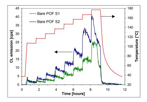
Figure 8.8: CL curves for the unexposed bare POFs S1 and S2.
