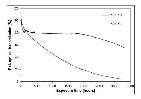
**Figure 8.6**: Optical transmission (averaged over three wavelengths) through POF cables S1 and S2, measured as a function of time during the exposure to the climate 92 °C / 95 %RH.
