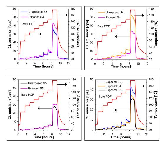
**Figure 8.37**: *CL curves for the unexposed and exposed bare POF samples S3, S4 and S5. The exposure condition was 90 °C / low humidity.*
