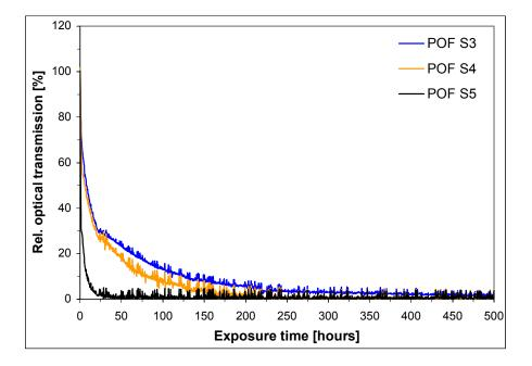
**Figure 8.25**: Optical transmission (averaged over three wavelengths) through bare POFs S3, S4 and S5, measured as function of time during the exposure to the climate 110 °C / low humidity.
