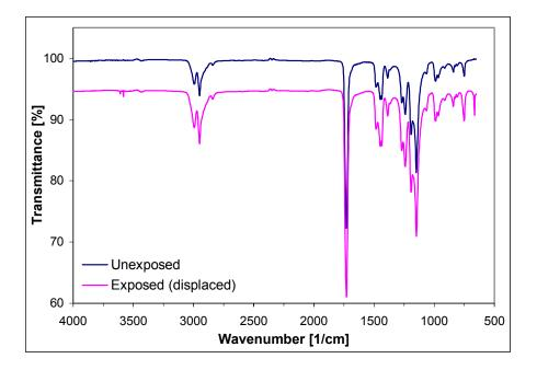
Figure 8.12: FTIR spectra of the unexposed and exposed core S2.
