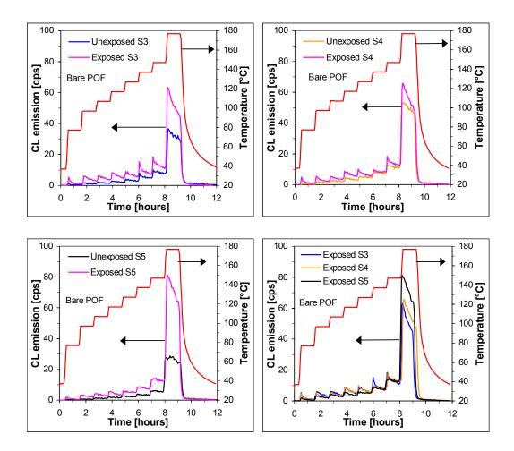
**Figure 8.35**: *CL curves for the unexposed and exposed bare POF samples S3, S4 and S5. The exposure condition was 100 °C / low humidity.*
