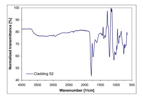
**Figure 8.16**: Difference IR spectrum (ATR-FTIR spectrum of the exposed minus unexposed cladding S2).
