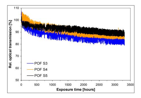
**Figure 8.28**: Optical transmission (averaged over three wavelengths) through bare POF sample S3, S4 and S5, measured as function of time during the exposure to the climate 90 °C / low humidity.
