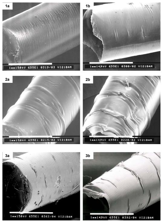
**Figure 8.22**: SEM photographs of the exposed POF (a) and cladding (b) of the sample S4: 1a & 1b. Exposed to 92 °C / 95 %RH; 2a & 2b. Exposed to 120 °C / low humidity and 3a & 3b. Exposed to 110 °C / low humidity.
