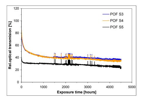
**Figure 8.26**: Optical transmission (averaged over three wavelengths) through bare POFs S3, S4 and S5, measured as function of time during the exposure to the climate 100 °C / low humidity.
