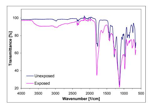
**Figure 8.14**: *ATR-FTIR spectra of the unexposed and exposed cladding S2*.
