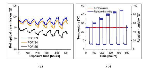
Figure 8.41: (a) Relative optical transmission through bare POFs, measured during the exposure to climates of steady room temperature with variable humidity; (b) Applied temperature and humidity scheme recorded during the exposure.
