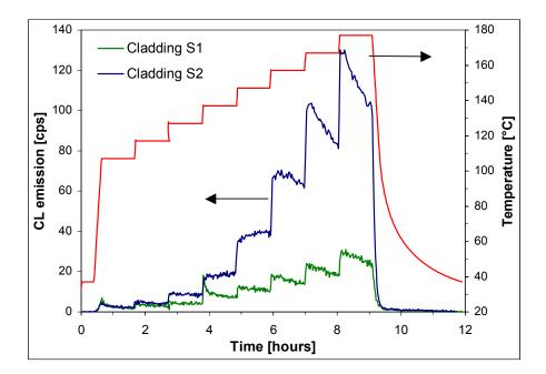
**Figure 8.9**: *CL curves for the unexposed claddings S1 and S2.*
