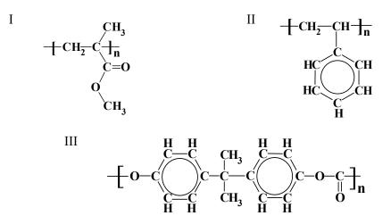
Figure 3.1: Molecular structure: (I) PMMA; (II) PS and (III) PC.
