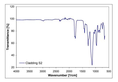
Figure 8.3: ATR-FTIR spectrum of the cladding S2.
