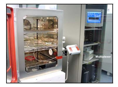
**Figure 7.2**: A photograph of an overview of the exposure test by using climatic chamber and multiplexer.
