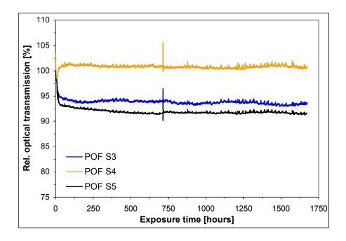
**Figure 8.24**: Optical transmission (averaged over three wavelengths) through the bare POFs S3, S4 and S5, measured as a function of time during the exposure to the climate 50 °C / 95 %RH.
