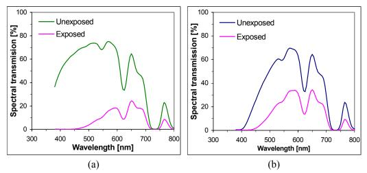
**Figure 8.20**: Spectral transmission of the unexposed and exposed POFs: (a) POF S1 and (b) POF S2.
