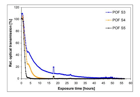
**Figure 8.21**: Optical transmission (averaged over three wavelengths) through bare POF S3, S4 and S5, measured as a function of time during the exposure to the climate 92 °C / 95 %RH.
