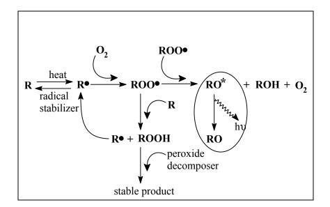
**Figure 6.3** *Autooxidation scheme for chemiluminescence in organic polymers.*
