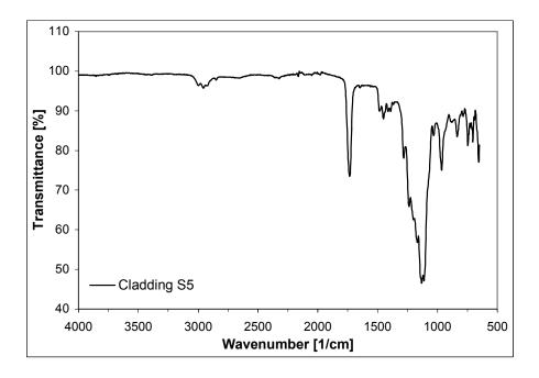
Figure 8.4: ATR-FTIR spectrum of the cladding S5.
