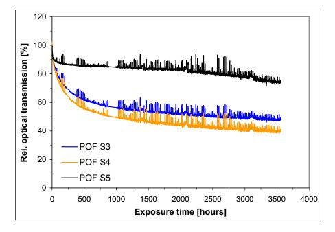
**Figure 8.23**: Optical transmission (averaged over three wavelengths) through the bare POFs S3, S4 and S5, measured as function of time during the exposure to the climate 92 °C / 50 %RH.
