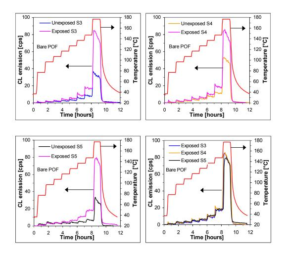
**Figure 8.33**: *CL curves for the unexposed and exposed bare POF samples S3, S4 and S5. The exposure condition was 92 °C / 50 %RH.*
