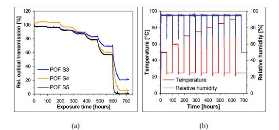
**Figure: 8.40**: *(a)* Relative optical transmission through bare POFs, measured during the exposure to climates of steady humidity and variable temperature; (b) Applied temperature and humidity scheme recorded during the exposure<sup>1</sup>.
