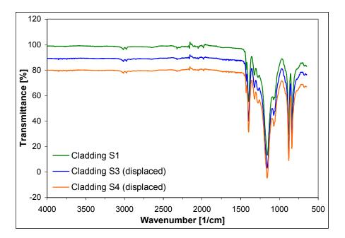
Figure 8.2: ATR-FTIR spectra of claddings S1, S3 and S4.
