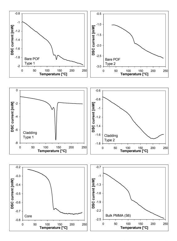
**Figure 8.1**: DSC second heating curves for bare POFs, claddings, core and bulk PMMA (S6).
