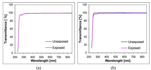
**Figure 8.18**: UV/visible transmittance spectra of the core: (a) sample S1 and (b) sample S2.
