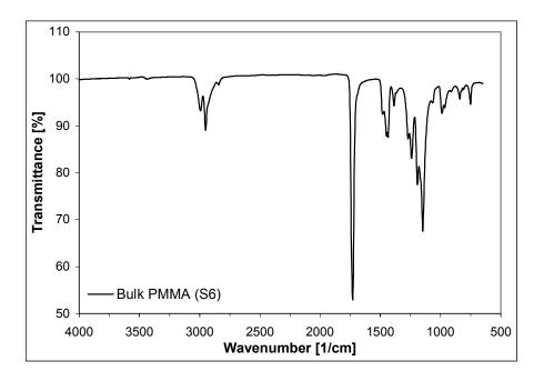
Figure 8.5: FTIR spectrum of the bulk PMMA (S6).
