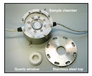
Figure 7.4: A photograph of an overview of the own built sample chamber.
