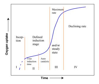
**Figure 5.2**: Schematic representation of the possible stages in the oxidative uptake history of polymer materials.
