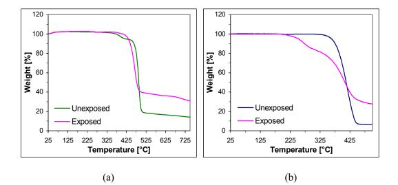
**Figure 8.17**: *Thermograms recorded under nitrogen atmosphere at a heating rate of 10 K min<sup>-1</sup> for: (a) cladding S1 and (b) cladding S2.*
