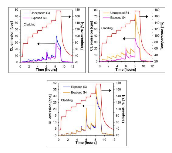
**Figure 8.36**: *CL curves for the unexposed and exposed cladding samples S3 and S4. The exposure condition was 100 °C / low humidity.*
