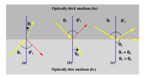
**Figure 2.1**: Schematic representation of the Snell's law of refraction and total internal reflection.
