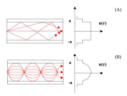
**Figure 2.3**: Scheme of the refractive index profile: (A) step-index optical fiber; (B) graded-index fiber.
