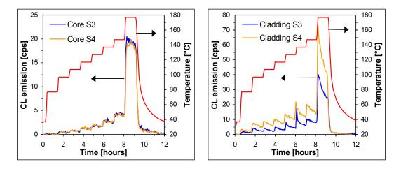
Figure 8.31: CL curves for the unexposed core and cladding of samples S3 and S4.
