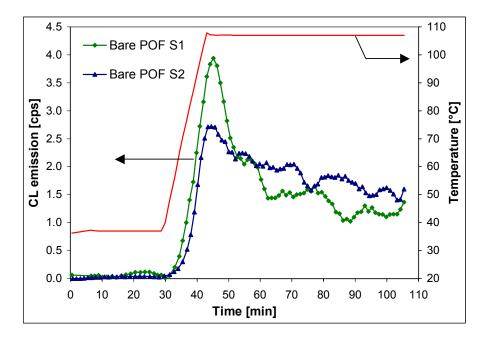
**Figure 8.7**: *CL emission curves (peak and plateau behavior) (at 107 °C) of the unexposed bare POF samples S1 and S2.*
